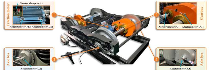
Figure 2. Test bed of train transmission systems.
